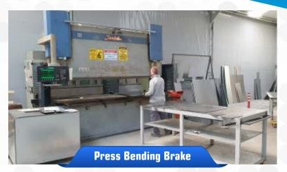
Cutting and bending steel, chrome-nickel, galvanized and aluminum plates between 1.2mm – 4mm in CNC controlled machines
